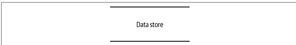
Figure 1-5. Data store symbols for drawing data flow diagrams
